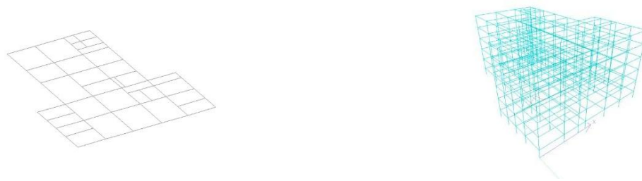
Figure 2: Importing STAAD Line Figure 3: An irregular grid used in the building's plan.
