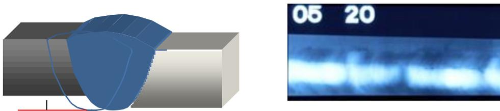
**Figure 12. Misalignment, or Hi-Low, and radiography film**
