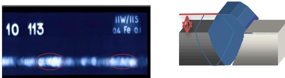
**Figure 7. Over weld metal and the image of radiography film**
