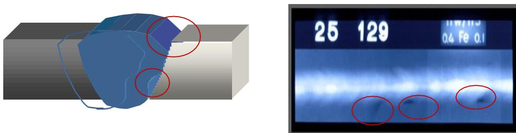
**Figure 13. Radiography film image with incomplete fusion**
