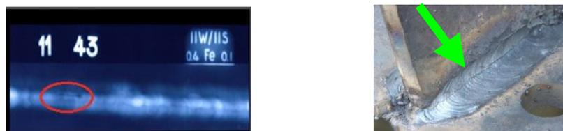
**Figure 2. Radiography film image of the longitudinal crack that has been**
