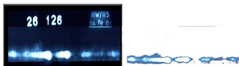
**Figure 24.** The radiography film image and the cluster of extra penetration
