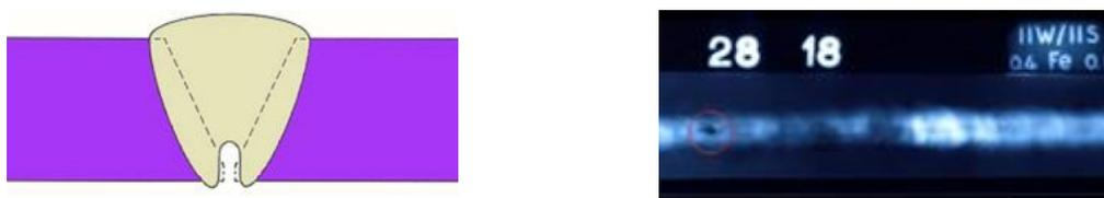
**Figure 9. The corresponding radiography film image of burn through**
