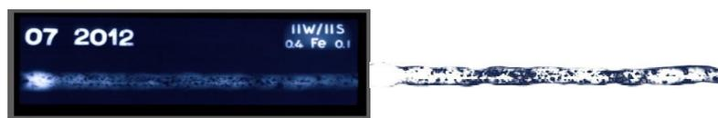
**Figure 19.** Image from radiography film and porosity cluster
