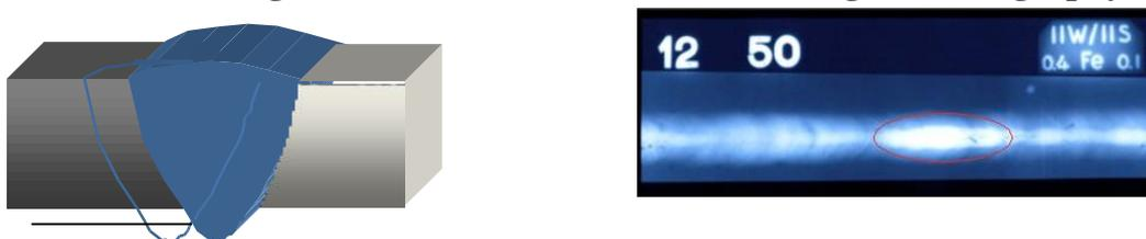
**Figure 8. The radiography film image of excess penetration**
