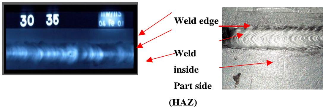
**Figure 14.** Part surface segmentation Based on the flaws and the appropriate radiography film
