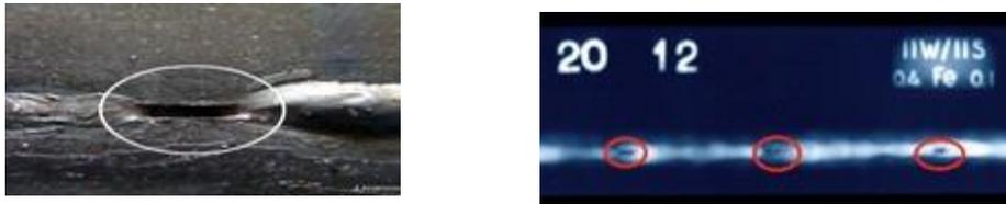
**Figure 5. Partial infiltration and associated radiography film image**
