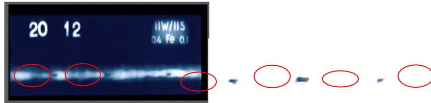
**Figure 25.** Picture from radiography film and missing penetration cluster
