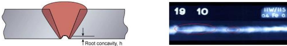
**Figure 10. Concavity of the weld root and associated radiography film picture**
