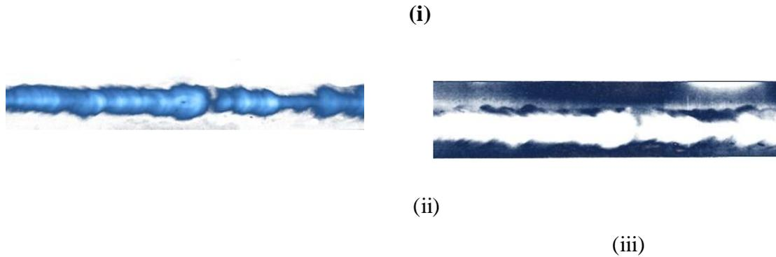
Figure 15. (i) Radiography film (ii) the weld inside cluster (iii) weld side clusterThe related normal clustering image and the defective weld portion are compared in order to discover the flaw. Two photos are subtracted in this section. The indexing of clusters is the following stage. An index of a cluster is produced for each area of the image that is input into the K-Means algorithm. Any area or group within the image is given a unique index in this stage.
