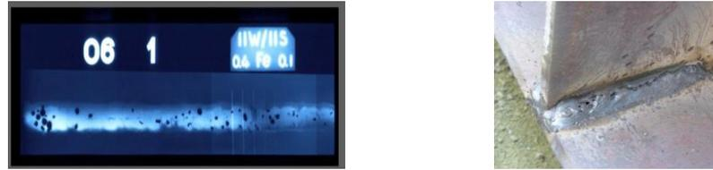
**Figure 3. Porosities in radiography film picture and fillet weld**
