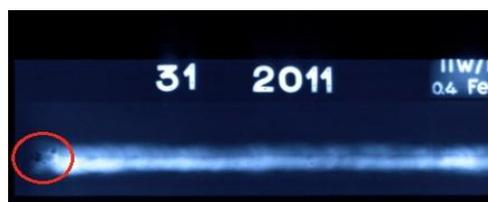
**Figure 4. The accompanying radiography film image defines the end crater and star crack.**
